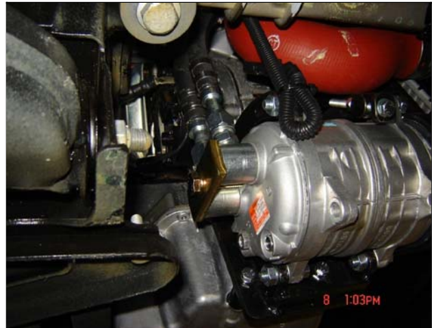
Figure 2-50 Fittings at Compressor
