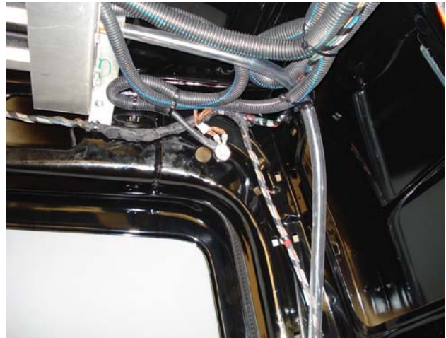
Figure 2-26 Electrical Harness Routing Roadside
