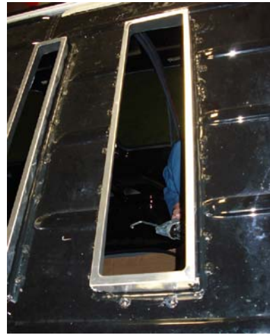
Figure 2-19 Transition and Rivets Sealed
