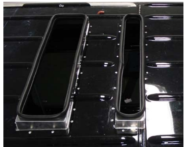
Figure 2-17 Transition Ducts Riveted
