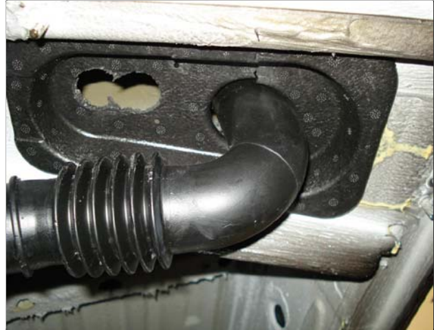
Figure 2-72 Plug Holes at Driver Column Underneath Vehicle
