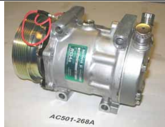
AC501-268A Compressor, TM-15, (6) Grv. Poly-V, 12 VDC, Direct Mt., Vertical O-Ring, With Fittings
