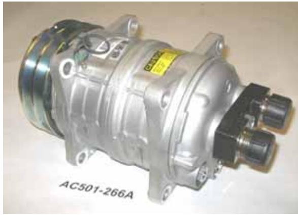
AC501-266A Compressor, TM-15, (2) "A" Grv., 12 VDC, Ear Mount, Horizontal Tube-O, With Fittings
