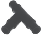
27-0102 Y-splicer 5/8" 43% fibreglass reinforced nylon 6/12. For 5/8 and 3/4" hose.
