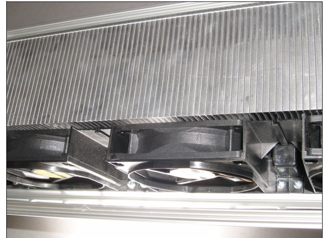
Close up view of convector and the axial fans
